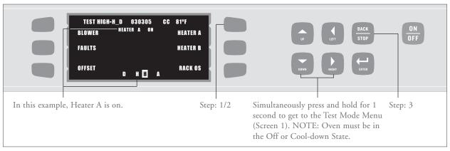
FIGURE 30: Checking Heater A
